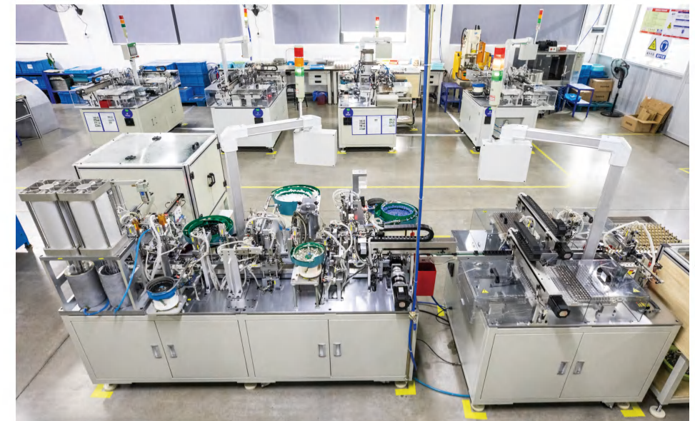
Solenoid valve Automatic Assembly Line
